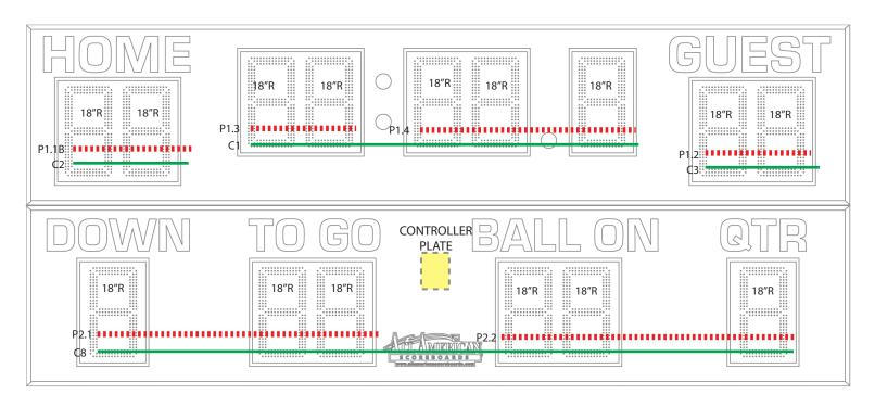
Power Supply Outputs (Full Brightness & Full Digits): P1.1≈2.92A P1.2≈2.60A P1.3≈1.93A P1.4≈290A P2.1≈3.57A P2.2≈3.57A
